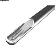
In sheathed thermocouples the flexible part of the probe consists of a mineral-insulated metal-sheathed cable (MIMS cable). It features a metal outer sheath, which contains the insulated internal leads, embedded within a high-density ceramic compound. Sheathed thermocouples, due to their flexibility and the small diameters that are possible, can be used in areas that are difficult to access.
