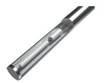
In sheathed resistance thermometers the flexible part of the probe consists of a mineral-insulated metal-sheathed cable (MIMS cable). It features a stainless steel outer sheath, which contains the insulated internal leads, embedded within a high-density ceramic compound. The measuring resistor is connected directly to the internal leads of the sheathed cable.
